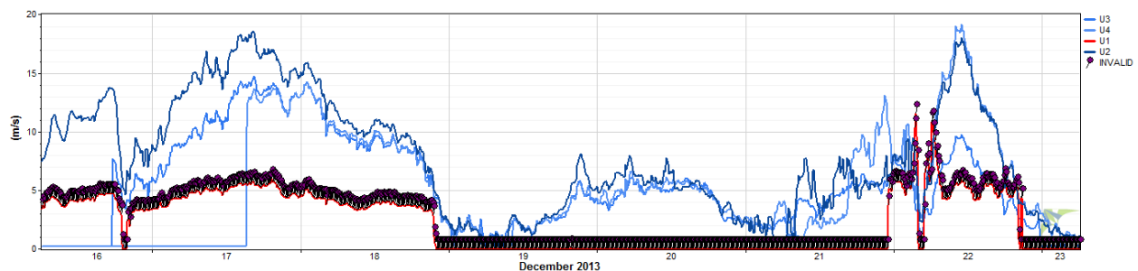
Figure 4-7 - After 2013-Dec-12, while D1 was erratic, U1 consistently underperformed and was flagged invalid
