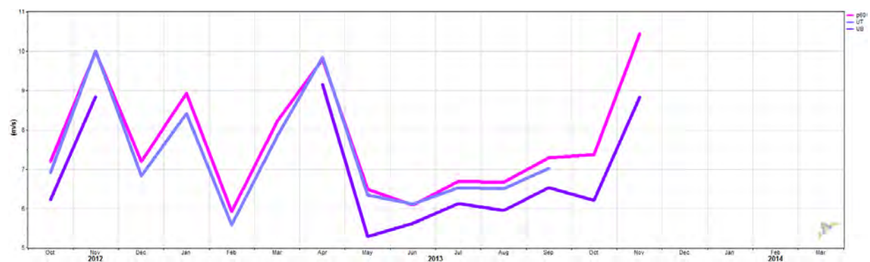
Figure 8-19 - Monthly Hub height (pink) and UT (blue) and UB (purple) wind speeds with recovery threshold for averaging relaxed to 40%
