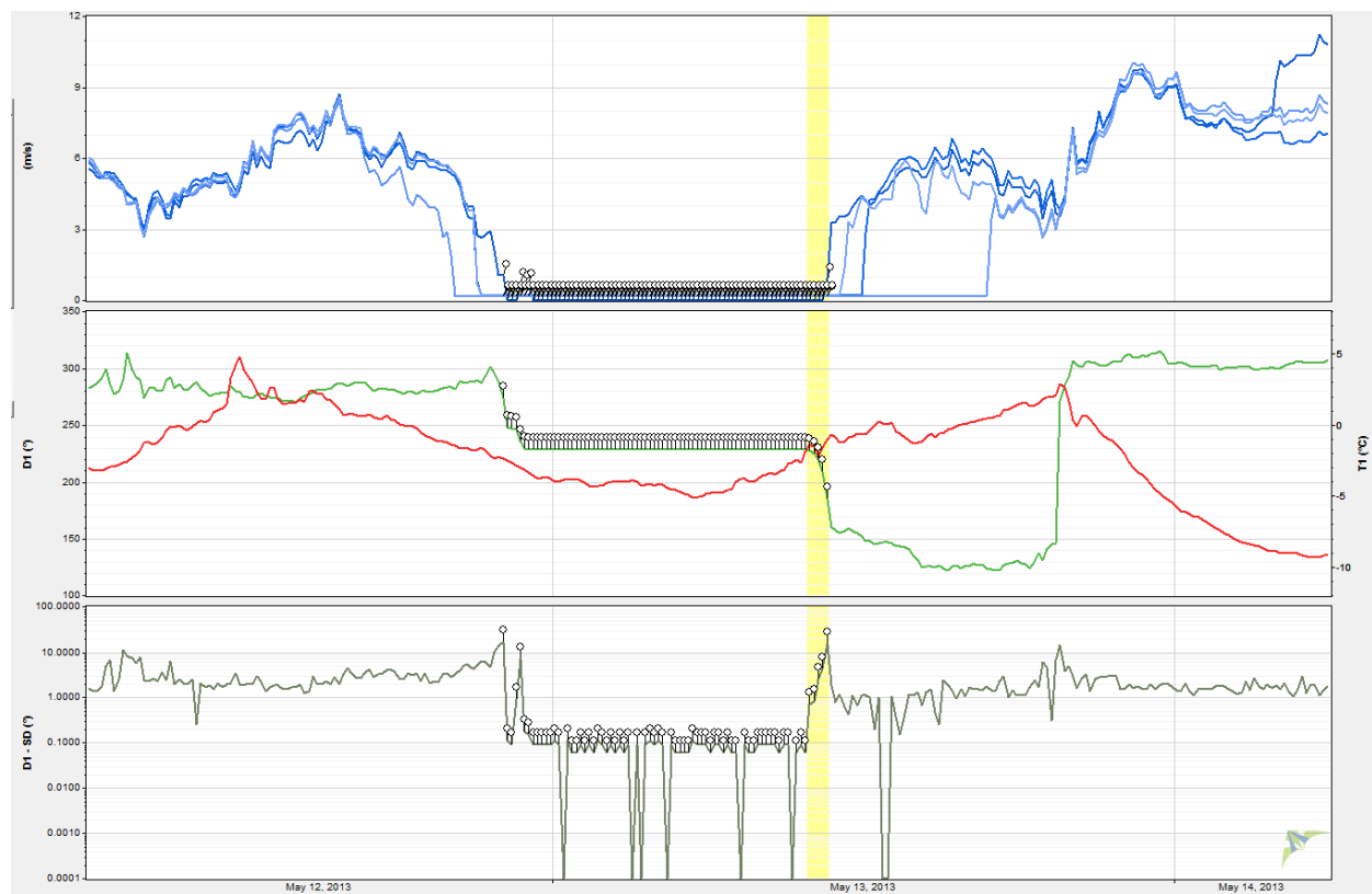
Figure 4-11 - Obvious case of an extended period of D1 icing and corresponding anemometer stalling Top: all anemometers stalled or slow (was also independently flagged) Middle: D1 flat-line indicating vane stalling, T1 low Bottom: D1-SD very low
