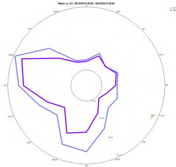
Figure 7-7 - Mean wind speed roses, 2012-10-5 to 2013-10-04 UT blue, UB purple
