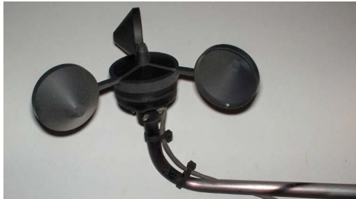
Figure 3: An anemometer is a piece of scientific equipment that measures wind speed. These are placed on the wind monitoring tower shown in Figure 4.
