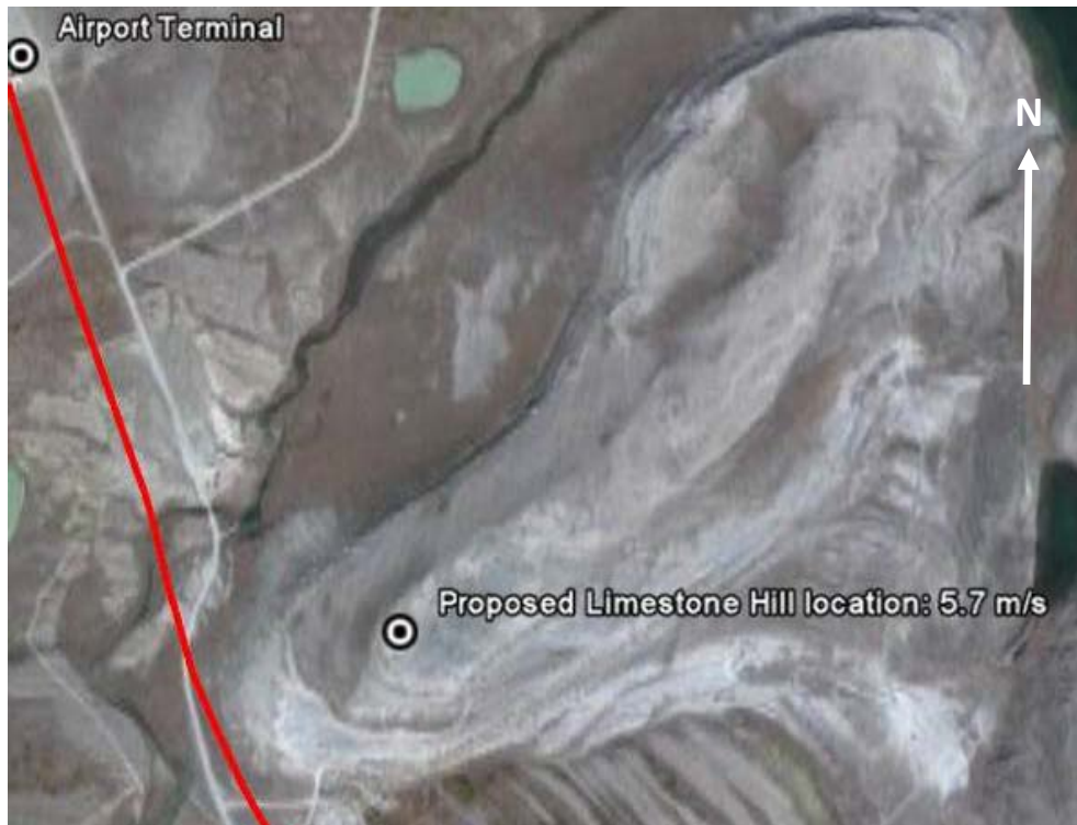
Figure 5: Limestone Hill proposed wind turbine location. The long-term annual average wind at this site is 5.7 metres per second (20.5 km/h) at 37 metres above ground. The red line is the power line which runs to about 400 metres from the site. The image is from Google Earth.
