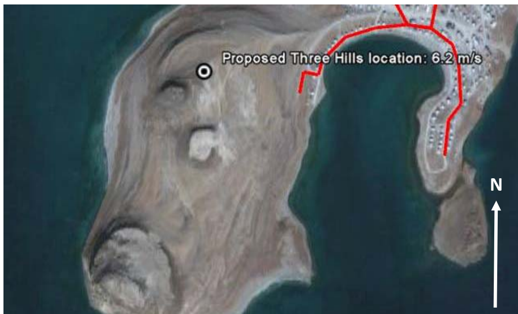
Figure 6: Three Hills proposed wind turbine location. The long-term annual average wind at this site is 6.2 metres per second (22.3 km/h) at 37 metres above ground. The red line is the power line which runs to about 400 metres from the site. The image is from Google Earth.
