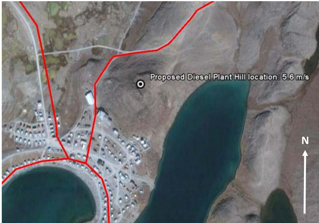
Figure 7: Hill behind the Diesel Plant. The long-term annual average wind at this site is 5.6 metres per second (20.2 km/h) at 37 metres above ground. The red line is the power line which runs to about 160 metres from the site. The site is also 325 metres from the diesel plant. The image is from Google Earth.
