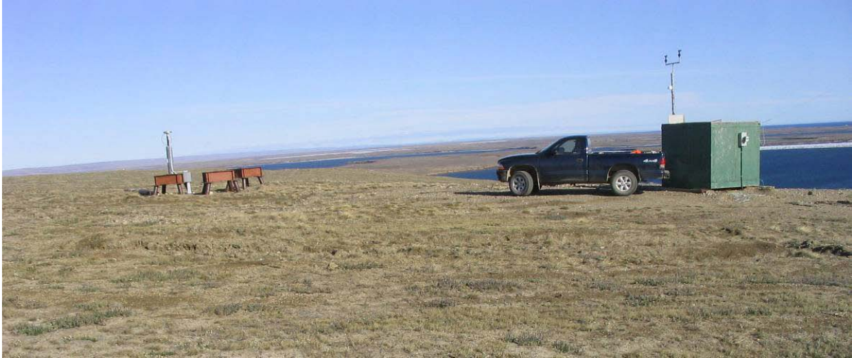
Figure 4: Site of the old wind turbine. The turbine foundation is to the left. The wind monitoring station here has heated wind sensors mounted on a post attached to the green hut on the right side of the photo.
