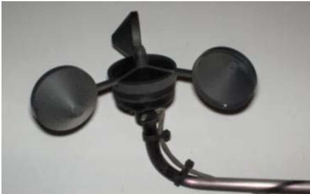
Figure 2: An anemometer is a piece of scientific equipment that measures wind speed. These are placed on the wind monitoring tower shown in Figure 3.
