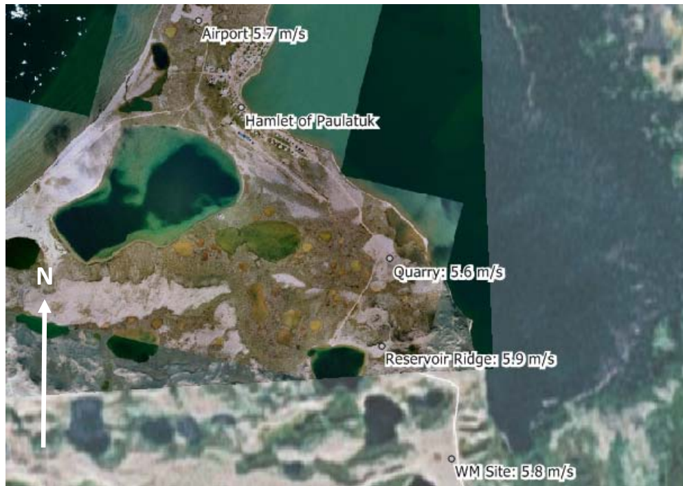
Figure 4: Paulatuk area showing the location of the wind measurements and the possible wind developments (Quarry and Reservoir Ridge). Images are from MACA and Google Earth.
