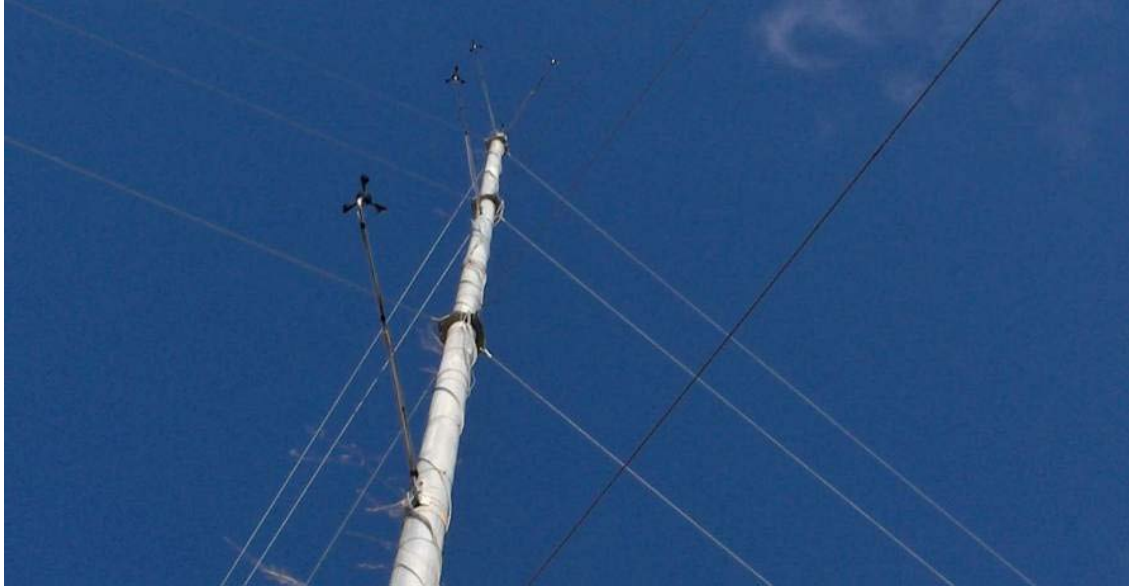
Figure 5: Looking up at the ARI wind monitoring station set up at site WM #2. The anemometer booms are pointing to the southwest.
