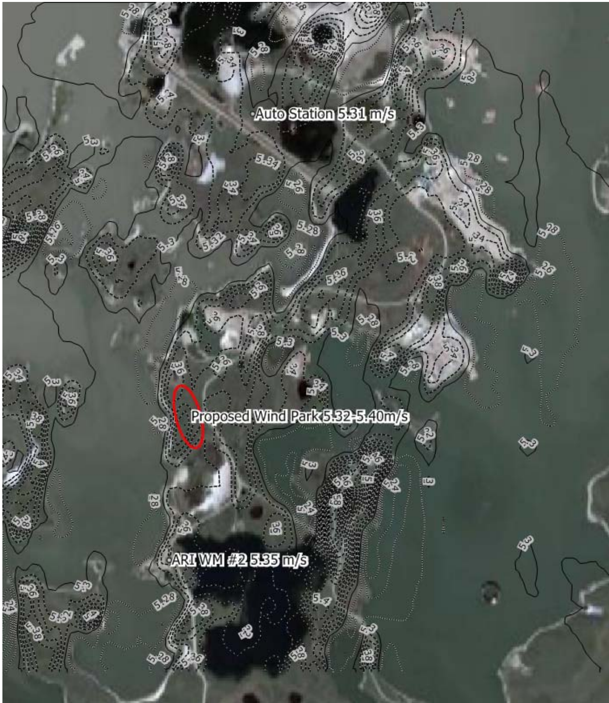
Figure 11: Tuktoyaktuk mean wind speed contours based on the numerical model MS-Micro. The wind speeds are modelled at 37 m AGL. The contour interval is 0.02 m/s. The black solid line is 5.3 m/s, the dotted lines are below 5.3 m/s, and the dashed lines are above 5.3 m/s. The sites are labelled with wind speeds estimated from the model.
