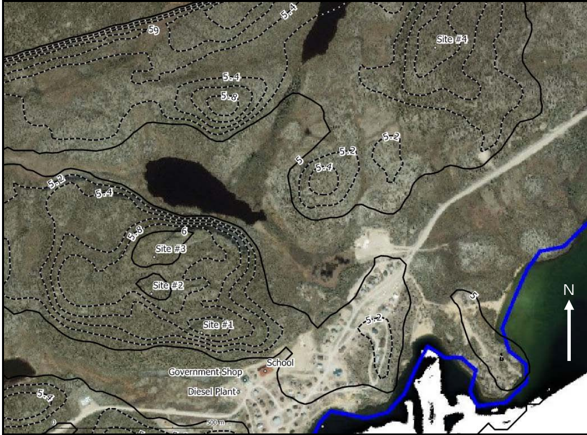
Figure 2: Aerial image of Wekweeti overlaid with wind speed contours. No contours are shown for the areas with wind speeds below 5m/s and the contour interval is 0.2m/s.
