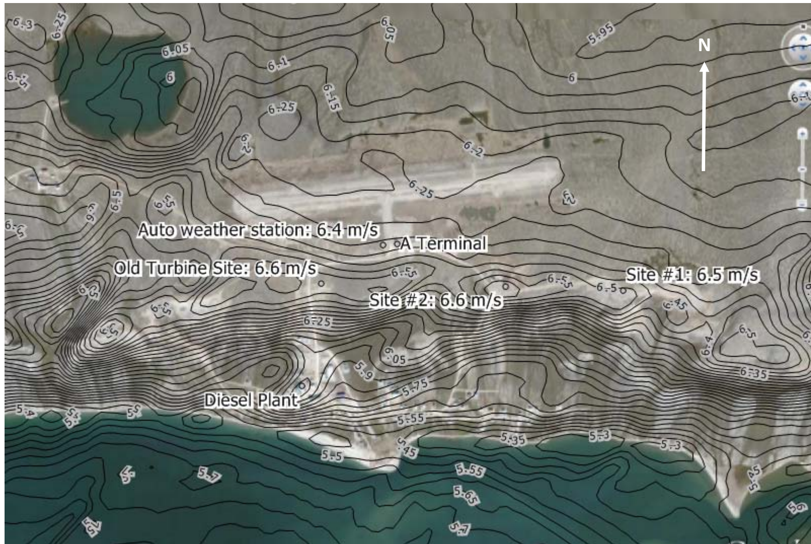
Figure 11: Mean wind speed contours based on the numerical model MS-Micro. The wind speeds are modeled at 37 m AGL. The contour interval is 0.05 m/s. The sites are labelled with wind speeds estimated from the model. Image is from Google Earth.
