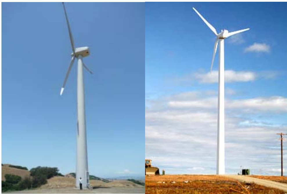
Figure 3: The two wind turbines considered in the economic study for Norman Wells. On the left is the Aeronautica A225 (225 kW) and on the right is the NorthWind 100 (100 kW).
