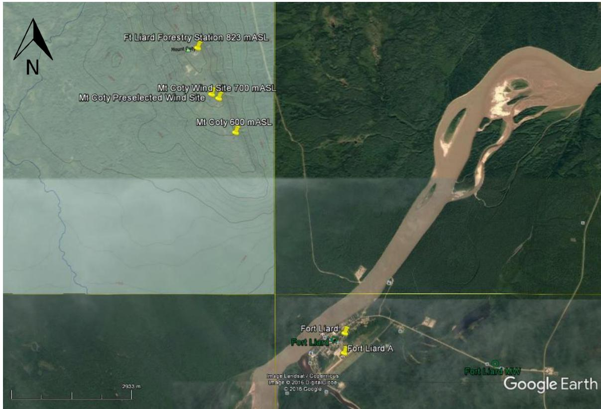
**Figure 3: Map of Fort Liard and area showing Mt Coty and the Liard Highway. The Fort Liard Airport is next to the community and the weather station is indicated by “Fort Liard A”. Mt Coty sites include the preselected GNWT site, and sites used in wind modelling at 600 m ASL and 700 m ASL.**
