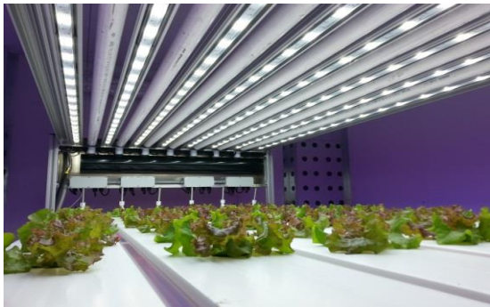
Figures 5-8: Top left displays the prototype modular production system with 3 levels of LED arrays displaying a range of capabilities for deploying different spectral qualities of light.
