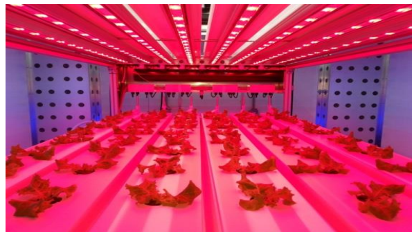
Figures 5-8: Top left displays the prototype modular production system with 3 levels of LED arrays displaying a range of capabilities for deploying different spectral qualities of light.
