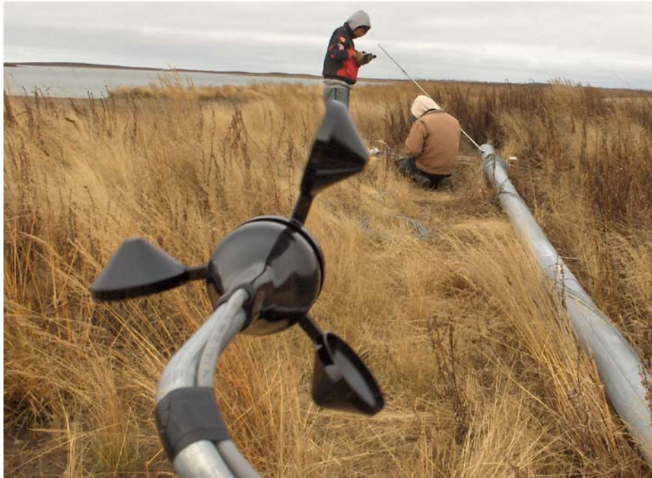
Figure 2: An anemometer (shown here in the foreground) is a piece of scientific equipment that measures wind speed. These are placed on the wind monitoring tower shown in Figure 3.
